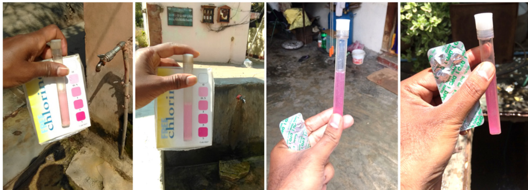
Figure 5: Field Testing of Residual Chlorine Using DPD – Rapid Tablets
